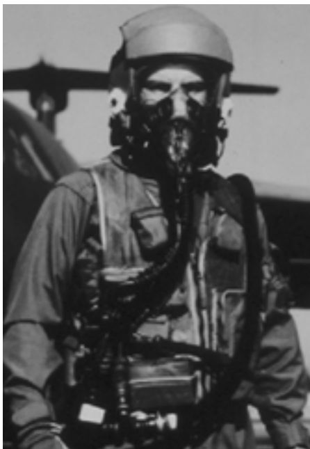
Fig. 16-11. The MBU-19/P Chemical–Biological Aircrew Mask. Reprinted from Brletich NR, Tracy MF, Dashiell TR. Worldwide NBC Mask Handbook . Edgewood, Md: Chemical Warfare/Chemical and Biological Defense Information Center; September 1992: 395.
